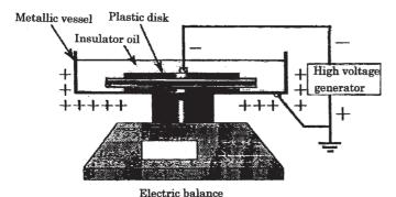
Fig. 1 Schematic diagram of the experiment.
