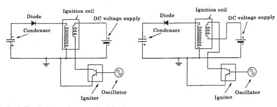
Fig. 3 Circuit diagram for generating AC pulses.
