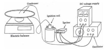
Fig. 2 Experimental set-up for the experiment.
